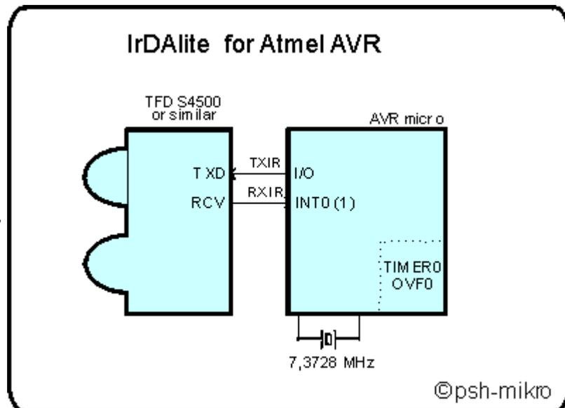
The IrDA Lite was developed for simple electronic devices with small system resources. For IrDA lite does not exist a defined specification. A Lite implementation can range from a minimum Lite up to a complete IrDA implementation. IrDA Lite is compatible with a fully implemented IrDA stack
