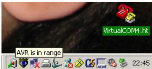
To get a IrCOMM connection you must have running a program like hyperterm that accesses the COM emulation of IrCOMM. For virtual COMM driver for winXP see: <http://www.ircomm2k.de/>
